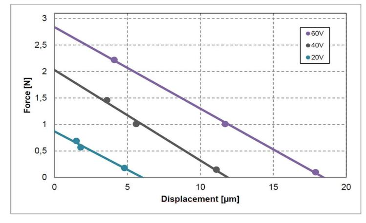
TDK PowerHapTM 0904H014V060 force-stroke diagram with different load springs. Typical stiffness 150 N/ mm. Source: 0904H014V060 Datasheet
