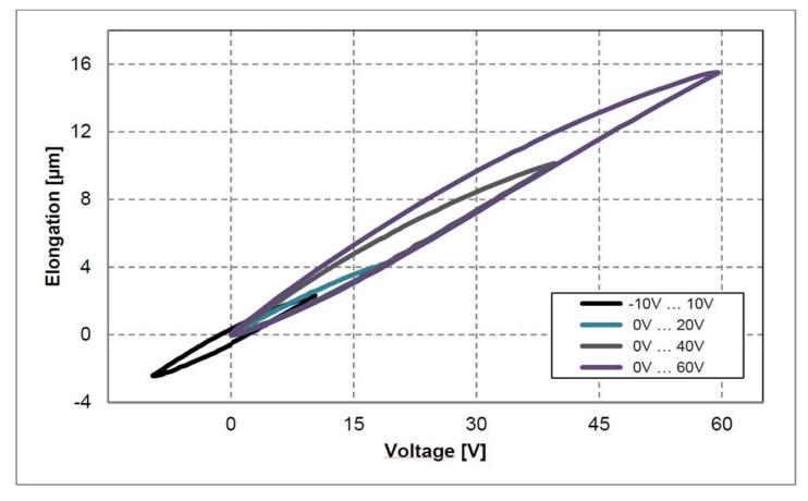
TDK PowerHapTM 0904H014V060 elongation measured between cymbal end-caps as a function of voltage. Source: 0904H014V060 Datasheet
