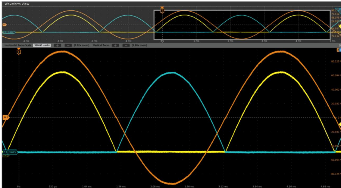
Figure 28: Optimized waveform. Crossings near zero are clean, waveform shows no sign of instability, top section of the waveform tracks well the desired sine waveform. Yellow: OUT+, Blue: OUT-, Orange: OUT - OUT-
