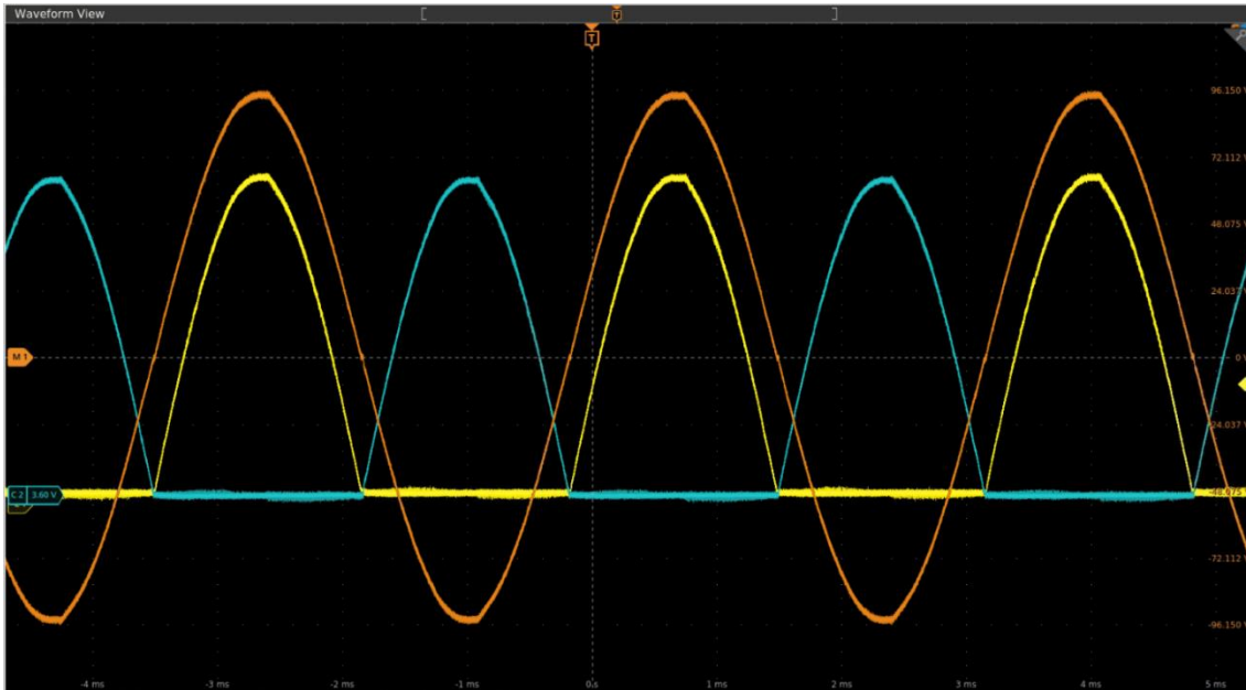
Figure 26: Example of a waveform with PARCAP too high
